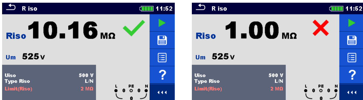
Figure 7.9: Examples of Insulation resistance measurement result
