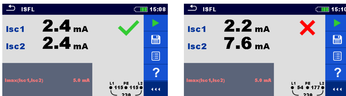
Figure 7.92: Examples of First fault leakage current measurement result
