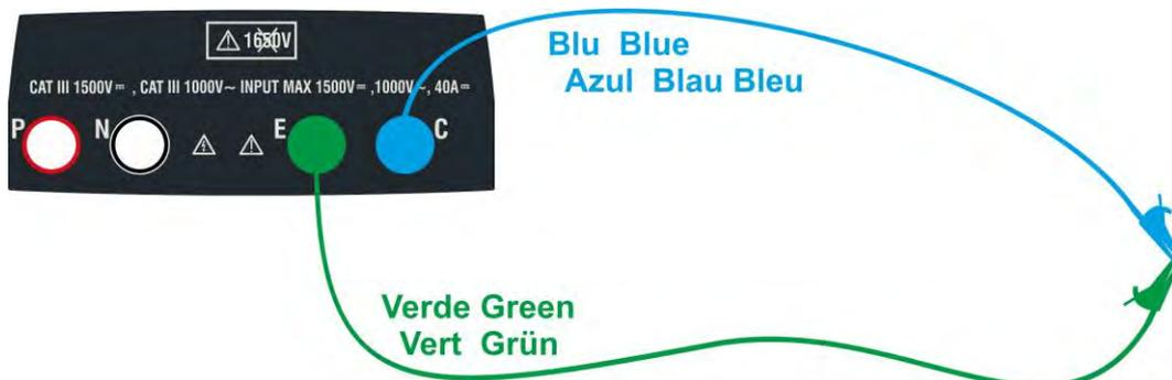
Fig. 5: Compensation of the measuring cables resistance
