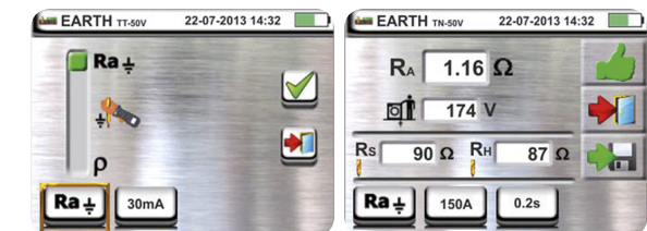
Earth resistance measurement by Volt-ampere method
