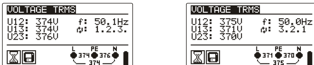
Figure 5.4: Examples of voltage measurement in three-phase system
