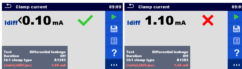
Figure 6.74: Examples of Clamp current measurement results
