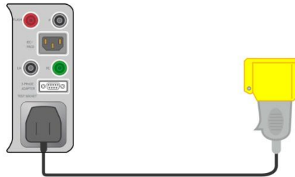
Figure 9.2: Connecting 110 V Test Adapter (A 1474)
