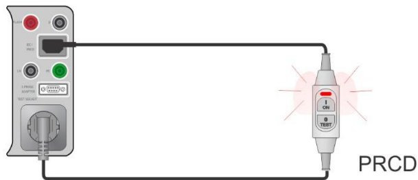
Figure 6.62: Open conductor (PRCD) test
