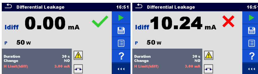
Figure 6.39: Examples of Differential Leakage measurement results
