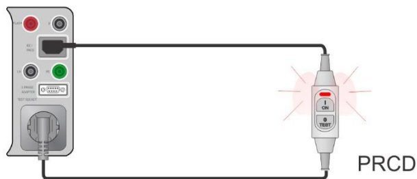
Figure 6.59: PE conductor (PRCD) test
