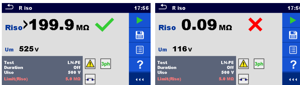
Figure 6.76: Examples of Insulation resistance (welding equipment) measurement results
