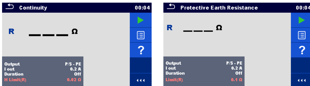
Figure 6.16: Continuity test // Protective earth resistance menu
